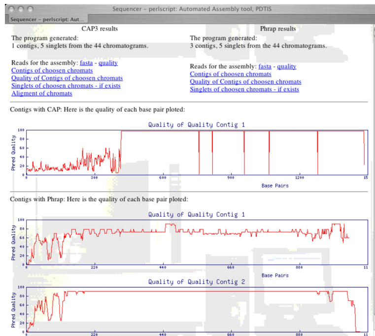
Figure 4. Assembly view. The user can select which sequences should be entered in the assembly process. New chromatograms can be included. The assembly is done with CAP3 and Phrap . The result files for the singlets and contigs are in FASTA format and the alignments are in text format. Furthermore, a quality graph is included, which shows the resulting Phred quality of each base pair in the contigs. With these chromatograms, Phrap and CAP3 generate different results.
